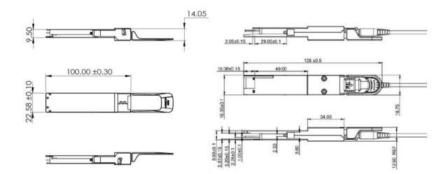
400G QSFP-DD to OSFP(RHS) Active Optical Cable (AOC) WS-D4O4-AOCxCxx4
